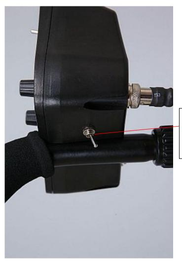
SEARCHMODE TRIGGER: 2-TONE Mode (only active with the mode trigger on the face plate set to FULL ALL)
